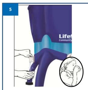
Water will now flow into the clean water tank. Open any of the four taps to collect and drink purified water.
