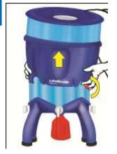
Pull the red lock and lift the upper part off of the safe water tank. Make sure to place it on a clean surface.
