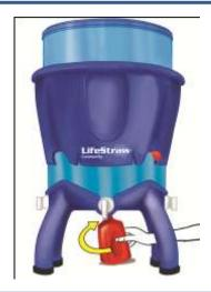
Put the backwash bottle back in its position. It should be in the center of the filter.
